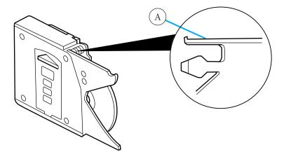
If you pull too hard on the disc holder, the disc holder may come completely out of the magazine. If this happens, reinsert the disc holder back into the magazine while pressing on the lever (A).
